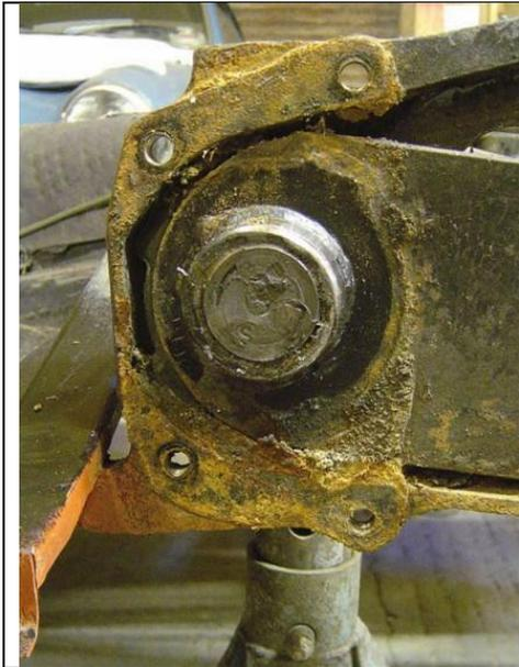
Here is a photo of how the spring plate looks once you've removed the covers and the outer rubber bushes. Remember to mark the current position so you can revert back if need be but also so you can count the amount of splines you're adjusting by.
